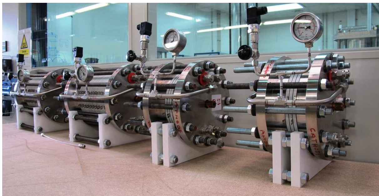
Electrolyser stacks (Source: ITM Power)
